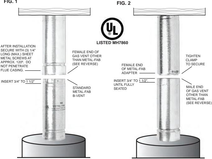
Metal-Fab round B-Vent has been evaluated and listed to Underwriter's Laboratories, Inc. to mate with other specifically identified and UL Listed round gas vent, in 3" through 6" diameters. Metal-Fab's approval covers connections to the following B-Vent products:
