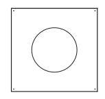
Used when pipe is supported by the TGAS. The oval I.D. of this plate covers any gap left between the chimney pipe and the ceiling. Select the plate which corresponds with the ceiling pitch. I.D. sized to fit over trim sleeve (TGTS).
