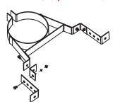
Enables adjustment of standard wall band (TGWB) from 2" - 6"
