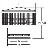
This cap is similar to TGC, but is produced without twist locking buttons. Cap slips onto pipe and is attached with packaged screws. Easily removed for cleaning. See TGC size chart.
